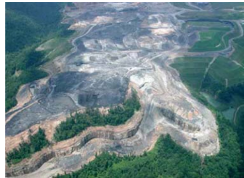
An example of mountaintop removal for coal mining
